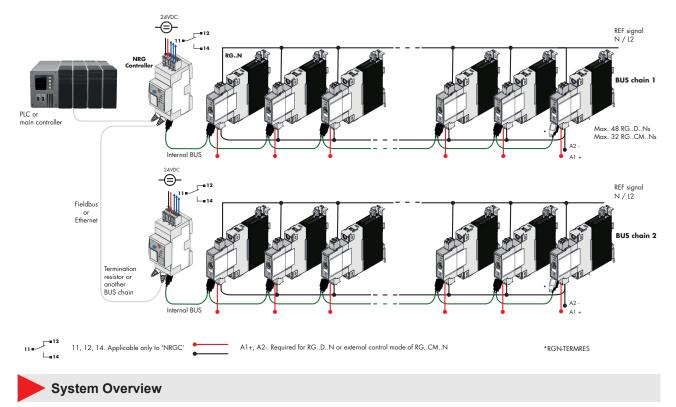
The NRG is a system consisting of one or more BUS chains that enable communication between the field devices (such as the solid state relays) and the control devices (such as the machine controller or PLC).
