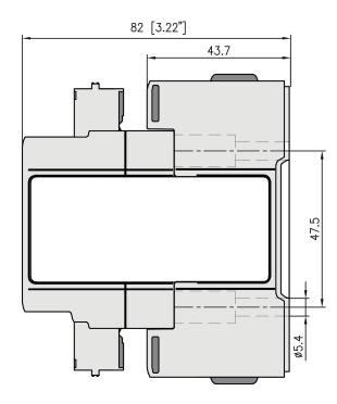
Housing width tolerance +0.5mm, -0mm as per DIN 43880. All other tolerances +/- 0.5mm. Dimensions in mm.
