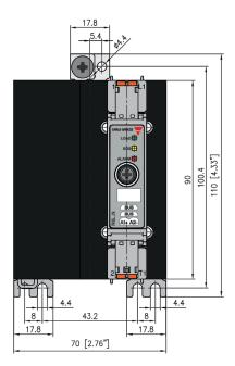
Housing width tolerance +0.5mm, -0mm as per DIN 43880. All other tolerances +/- 0.5mm. Dimensions in mm.
