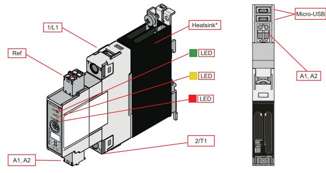
\* integrated for RGC..N versions. RGS..N do not have an integrated heatsink
