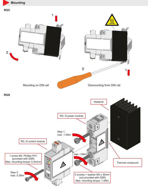
Step 1: Mount RG..N power module to Heatsink Step 2: Mount RG..N control module on RG..N power module
