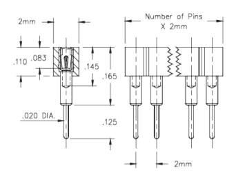
**Description:** Interconnect Socket Standard Solder Tail Socket Accepts .015"- .026" (0,38 - 0,66 mm) dia leads Single Row Through Hole
