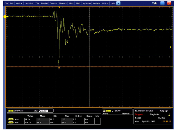
Figure 3. ESD Clamping Voltage Screenshot Negative 8 kV Contact per IEC61000-4-2
