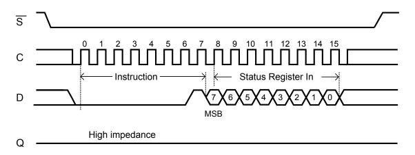
Driving the Chip select  $(\overline{S})$  signal high at a byte boundary of the input data triggers the self-timed Write cycle that takes  $t_W$  to complete (as specified in AC tables in Section 9 DC and AC parameters).
