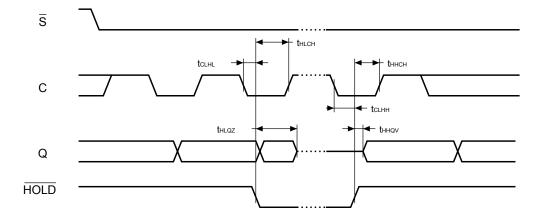
Figure 22. Serial output timing
