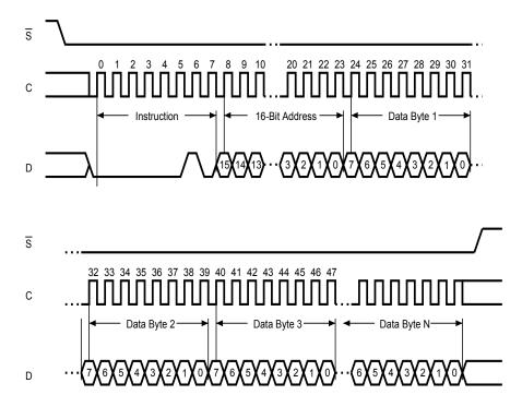
1. Depending on the memory size, as shown in Table 5. Significant bits within the address bytes, the most significant address bits are Don't care.
