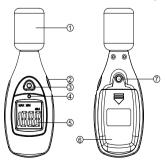
① Windscreen & 1/2 inch Electret Condenser microphone If you operate at wind speed over 10m/sec, please put protective accessories in front of the microphone.
