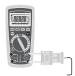
Note: The temperature probe is fitted with a type K mini connector.
