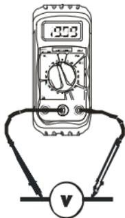
4. Read the voltage in the display. Reset the function switch to successively lower V DC positions to obtain
