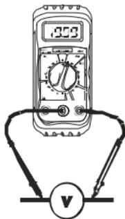
4. Read the voltage in the display. Reset the function switch to successively lower V AC positions to obtain a higher resolution reading. The display will indicate the proper decimal point and value.
