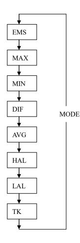
The infrared thermometer measures Maximum (MAX), **Minimum** (MIN). Differential (DIF), and Average (AVG) Temp. Each time you take a reading. This data is stored and can be recalled with the MODE button until а new is taken. measurement When the trigger is pulled
