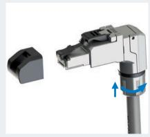
Step 5: Screw together cable strain relief
