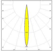
Dimensions: 35.0 mm x 35.0 mm Height: 15.00 mm ~12° smooth spot beam with 1.5 mm high location pins
