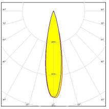
Dimensions: 35.0 mm x 35.0 mm Height: 15.00 mm ~25° medium beam with 3 mm high location pins
