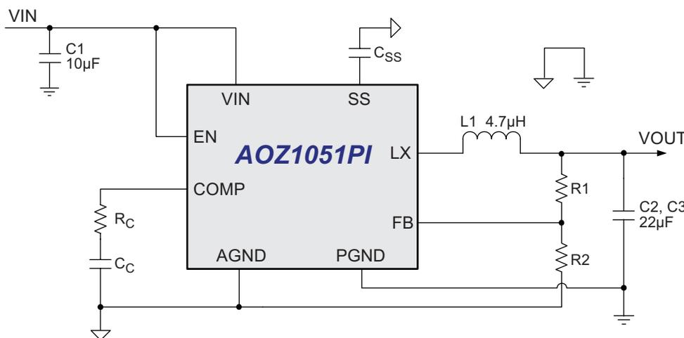
Figure 1. 3.3 V 3 A Synchronous Buck Regulator,  $F_s = 500$  kHz
