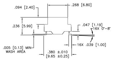
DIMENSIONS ARE IN INCHES [MILLIMETERS] WITH THE FOLLOWING TOLERANCES: [MILLIMETERS] ARE FOR REFERENCE ONLY. .XX=  $\pm$ .01 [ $\pm$ 0.25] .XXX=  $\pm$ .005 [ $\pm$ 0.13]
