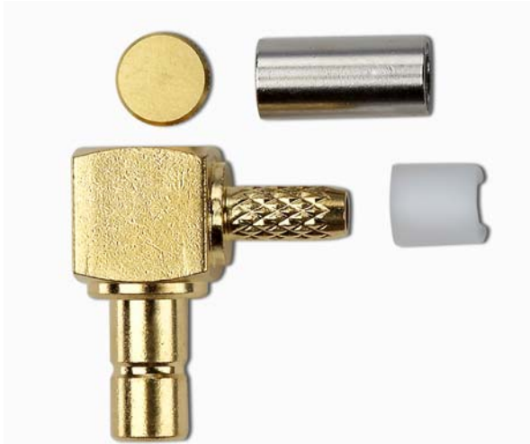
Model 72992 SMB JACK R/A CRIMP, RG174, 188, 316
