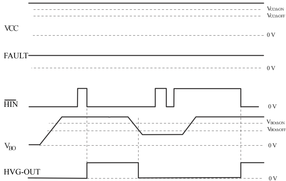
Figure 9. VBO Power-ON and UVLO timing
