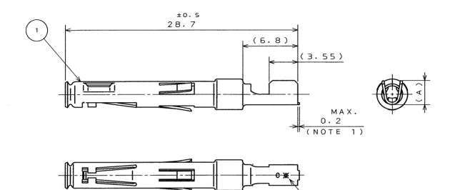
NOTE 1. NO PLATING ON THE SHEARED EDGES OF CONTACT.
