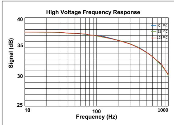
**FIGURE 2-20:** High Voltage Frequency Response: Signal vs Frequency ( $V_{PP} = 225\text{V}$ ,  $V_{CC} = 6.5\text{V}$ ,  $V_{LL} = 3.3\text{V}$ ,  $R_{BIAS} = 150\text{ k}\Omega$ ,  $V_{IN} = 0$  to  $2.98\text{V}$ , Load =  $0.22\text{ }\mu\text{F}$ ).
