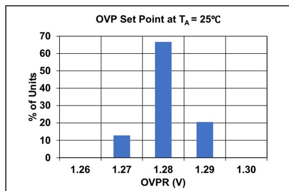
**FIGURE 2-6:** OVP Set Point Distribution at  $T_A = 25^\circ\text{C}$ .
