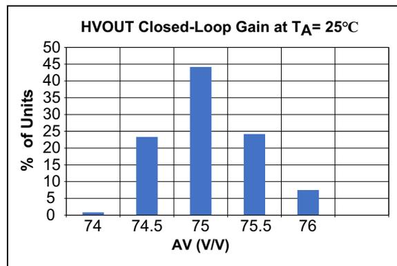
**FIGURE 2-19:** HVOUT Closed-Loop Gain Distribution at  $T_A = 25^\circ\text{C}$ .
