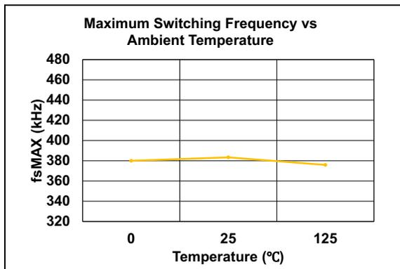
**FIGURE 2-2:** Maximum Switching Frequency vs. Ambient Temperature.
