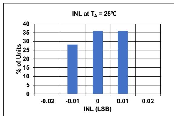
**FIGURE 2-11:** INL Distribution at  $T_A = 25^\circ\text{C}$ .
