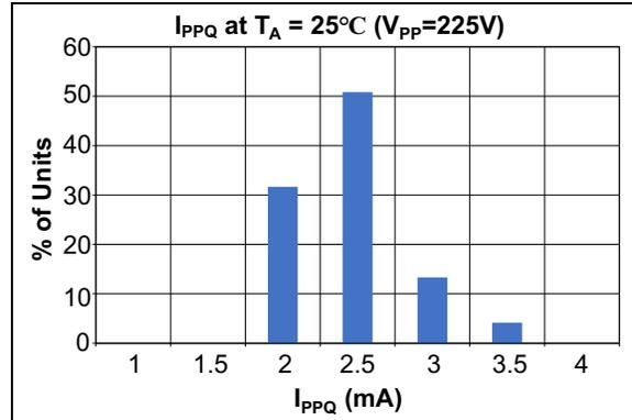
**FIGURE 2-17:**  $I_{PPQ}$  Distribution at  $T_A = 25^\circ\text{C}$ .
