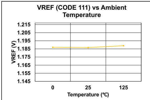
**FIGURE 2-7:**  $V_{REF}$  (Code 111) vs Ambient Temperature.
