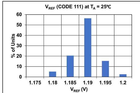
**FIGURE 2-10:**  $V_{REF}$  (Code 111) Distribution at  $T_A = 25^\circ\text{C}$ .
