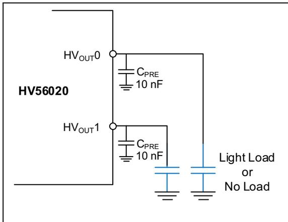
FIGURE 4-2: Preload Capacitors.
