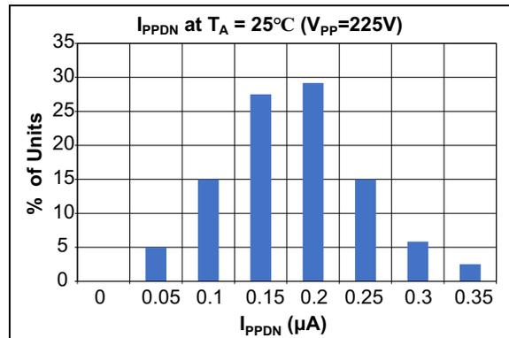
**FIGURE 2-18:**  $I_{PPDN}$  Distribution at  $T_A = 25^\circ\text{C}$ .
