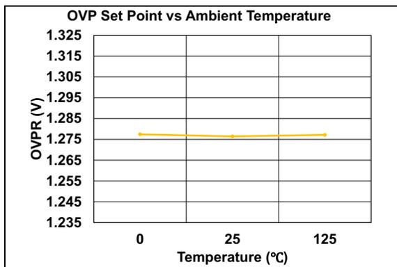
**FIGURE 2-3:** OVP Set Point vs Ambient Temperature.
