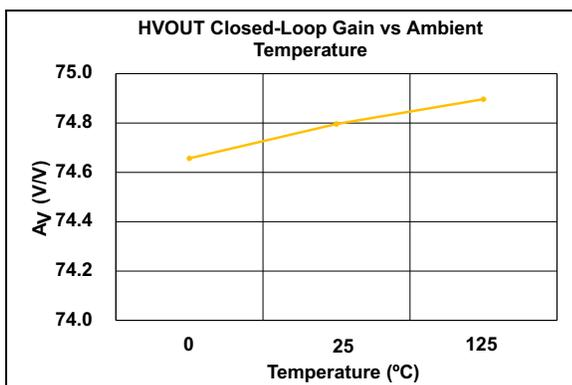
**FIGURE 2-16:** HVOUT Closed-Loop Gain vs Ambient Temperature.
