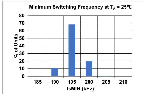
**FIGURE 2-4:** Minimum Switching Frequency Distribution at  $T_A = 25^\circ\text{C}$ .
