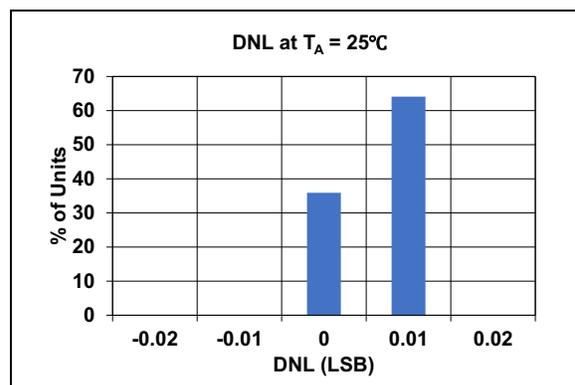
**FIGURE 2-12:** DNL Distribution at  $T_A = 25^\circ\text{C}$ .
