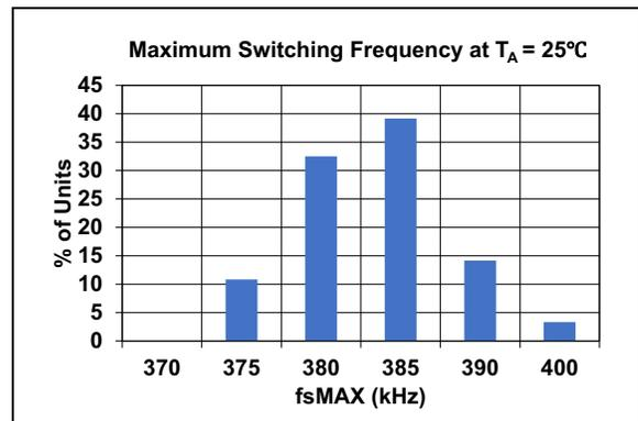
**FIGURE 2-5:** Maximum Switching Frequency Distribution at  $T_A = 25^\circ\text{C}$ .
