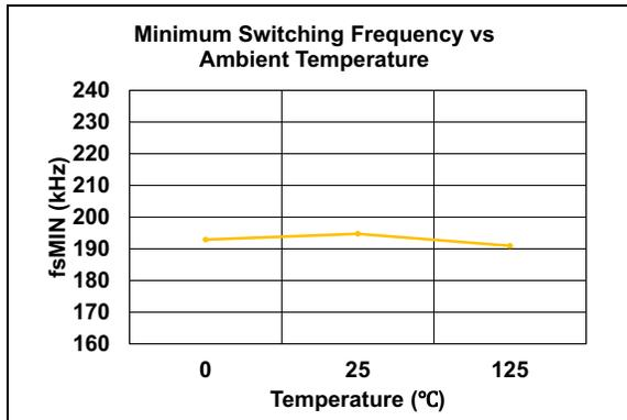
**FIGURE 2-1:** Minimum Switching Frequency vs. Ambient Temperature.
