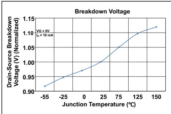
**FIGURE 2-22:** Breakdown Voltage.
