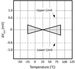
Figure 4: V<sub>OUT</sub> vs. Temperature (VRE102M)
