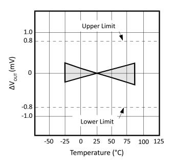
Figure 3: V<sub>OUT</sub> vs. Temperature (VRE102CA)
