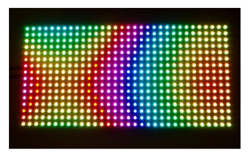
Of course, we wouldn't leave you with a datasheet and a "good luck!" We have a full wiring diagrams and working Arduino library code with examples from drawing pixels, lines, rectangles, circles and text. You'll get your color blasting within the hour! On an Arduino Uno or Mega, you'll need 12 digital pins, and about 800 bytes of RAM to hold the 12-bit color image (double that for the 32x32 matrix).
