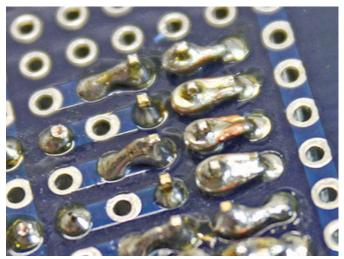
Depending on the make and model of proto shield, some pins are designed to connect in short rows.
