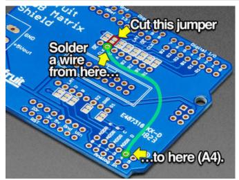
The shield requires a small modification to work with the Adafruit **Metro M4**:
