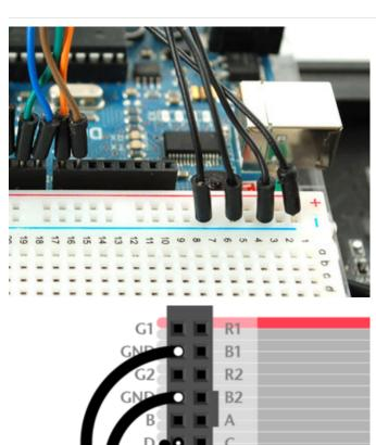
CLK OE **32x32** and **64x32** matrices require **three** ground connections. **32x16** matrices have **four**.
