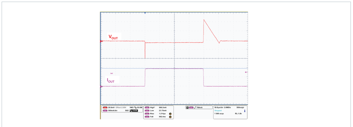
Figure 24. Load transient ( V_{IN} = V_{EN} = 3.5\text{ V} ; t_{RISE} = 1\text{ }\mu\text{s} ; I_{OUT} = 1\text{ mA} to 1\text{ A} )
