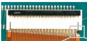
Incomplete FPC insertion
