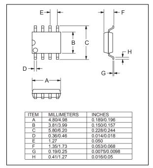
Figure 8. 8-pin SOIC package outline
