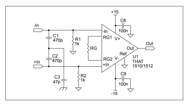
Figure 3. Basic 1510 / 1512 Circuit
