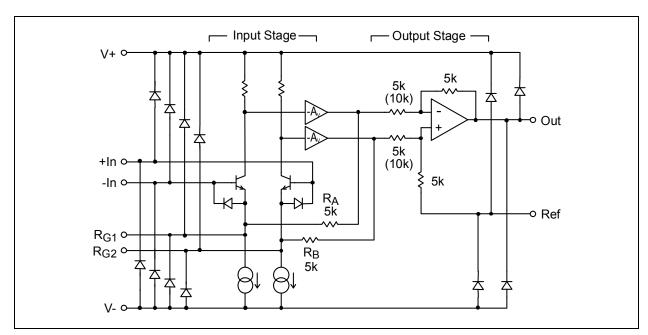
Figure 2. THAT 1510 / 1512 Equivalent Circuit with Protection Diodes
