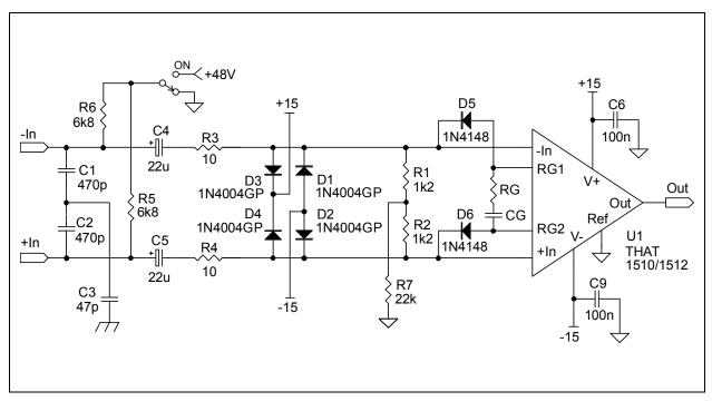
Figure 5. Recommended 1510 / 1512 Circuit with Phantom Power
