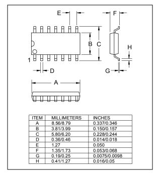
Figure 9. 14-pin SOIC package outline
