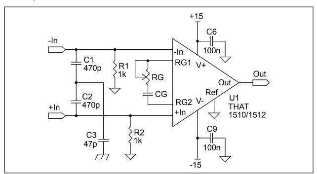
Figure 4. Basic 1510 / 1512 Circuit with Variable Gain
