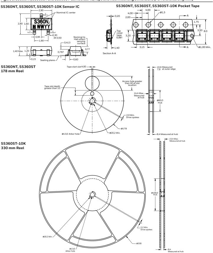
SS360NT, SS360ST, SS360ST-10K, SS460S, SS460S-T2, SS460S-T3, SS460S-LP
