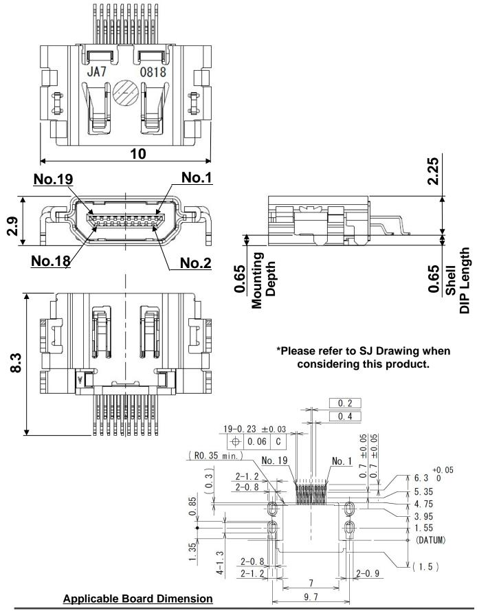
Receptacle --- On-board Type (shell 4 point DIP version) DC3RX19JA2 / 3 [SJ111288 / SJ111264]
