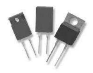
The MPT Resistor series are a range of T0220 and T0247 packaged, low inductance thick film power resistors. This small size, high power device with 5 models are ideally suited to applications where high power dissipation yet small size are key design requirements. The MPT Resistor series are the ideal solution for small snubber circuits, the output side of high speed pulse generators and low inductive resistor requirements in switch mode power supplies.
