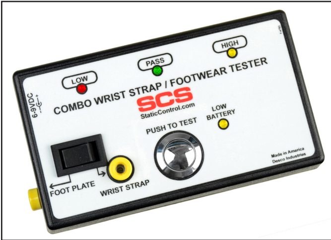
Figure 1. SCS 770030 Combo Tester
