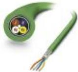
Network cable, PROFINET CAT5 (100 Mbps), 4-position, PUR halogen-free, green RAL 6018, shielded, free cable end, on free cable end, cable length: Free entry (0.5 ... 400 m), For drag chains
