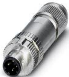
Data connector, PROFINET CAT5 (100 Mbps), 4-position, shielded, Plug straight M12, Coding: D, Push-in connection, knurl material: Zinc die-cast, nickel-plated, external cable diameter 4 mm ... 8 mm
