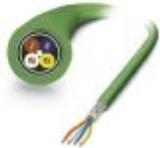
Network cable, PROFINET CAT5 (100 Mbps), 4-position, PVC, green RAL 6018, shielded, free cable end, on free cable end, cable length: Free entry (0.5 ... 400 m)
