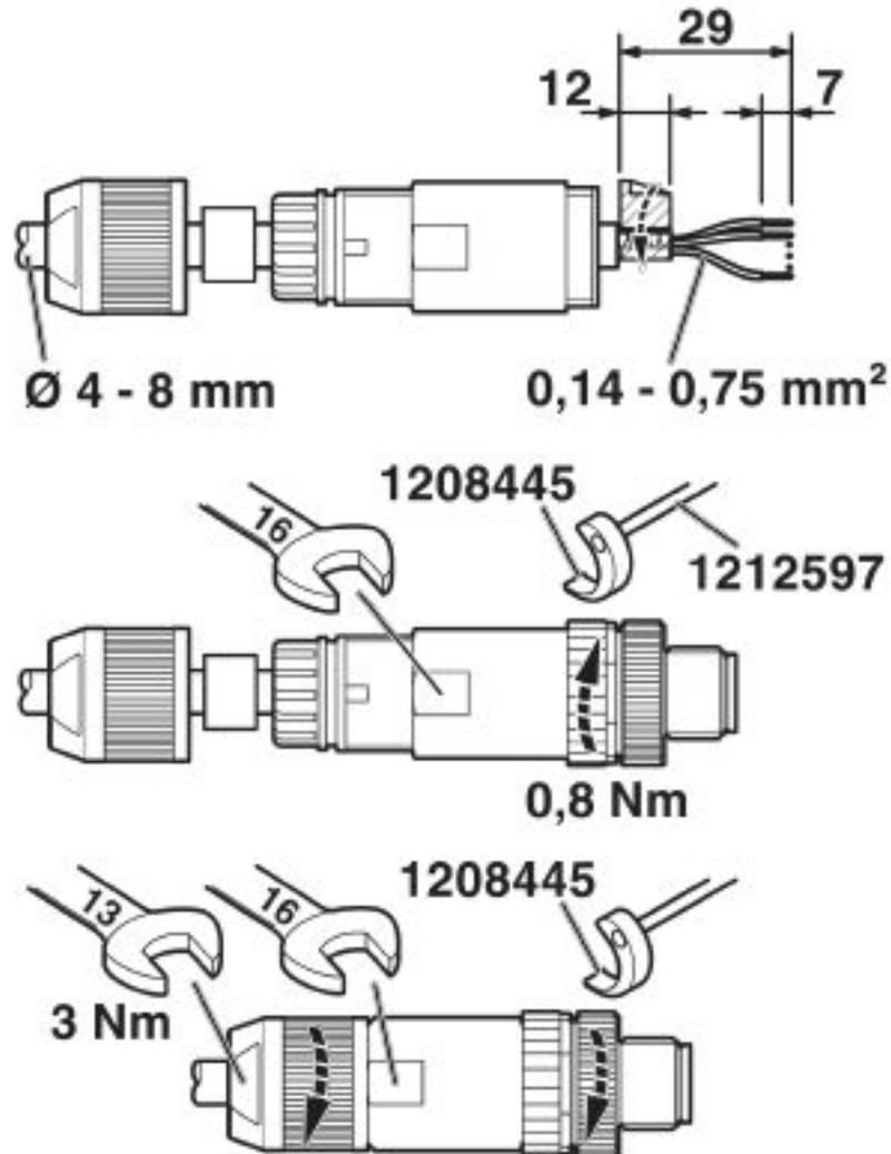
Slide the pressure nut and sleeve housing along the cable, strip the cable, shorten the shield, strip the single wires, connect the wires, in the case of a straight sleeve housing gently twist the wires together, stick the shielding foil around the shortened shield, in the case of a cable outside diameter  $< 6 \text{ mm}$  stick an additional shielding foil around the wire pack, screw the sleeve housing to the plug insert, screw the pressure nut tight.
