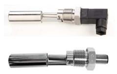
The SSF212 series are horizontally mounted switches that are fitted via a ½"NPT thread from the outside of the tank, so does not require access to the inside of the tank.
