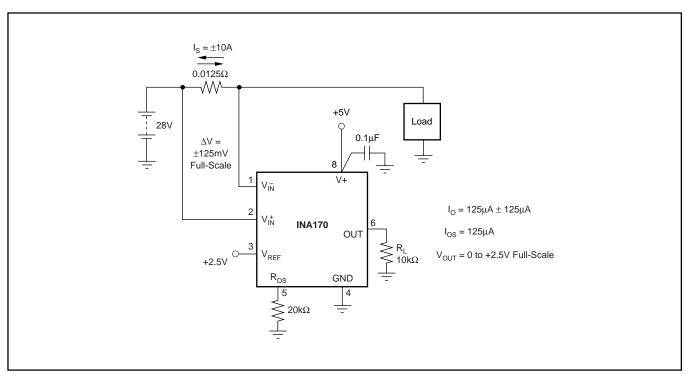
FIGURE 5. Bipolar Current Measurement.
