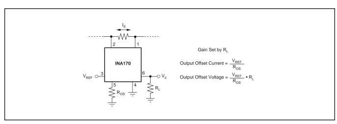
FIGURE 4. Offsetting the Output Voltage.
