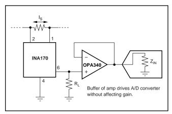
FIGURE 2. Buffering Output to Drive A/D Converter.
