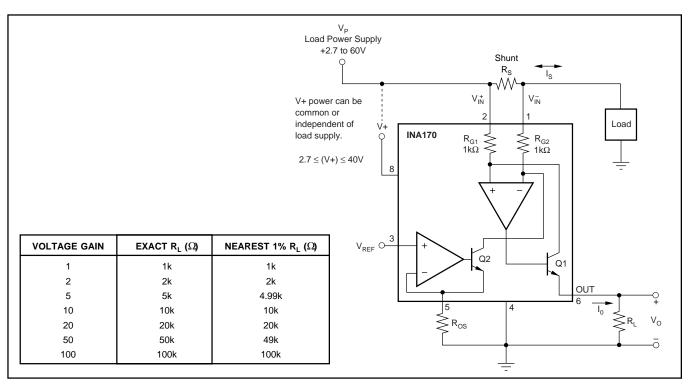
FIGURE 1. Basic Circuit Connections.
