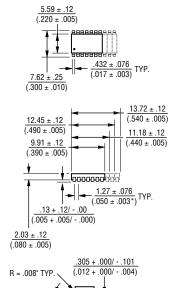
Lead coplanarity .102mm (.004 inch) max. at mounting surface.
