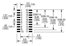
NOTE: Land pattern dimensions are based on design rules established by the Institute for Inter- $\!\mathbb{I}$ connecting and Packaging Electronic Circuits in [] IPC-SM-782
