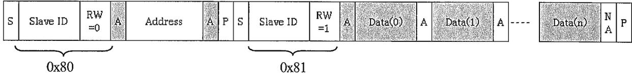
Data(0) is the register value which was assigned by Address. Data(1) and Data(2) are the register value of Address+1 and Address+2, respectively.
