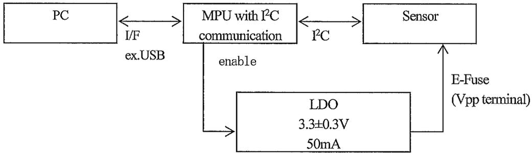
PC is used when different data is programmed to each sensor. It is unnecessary when same data which was set in MPU is programmed. Vpp terminal is on the back side of this sensor as shown in below figure.
