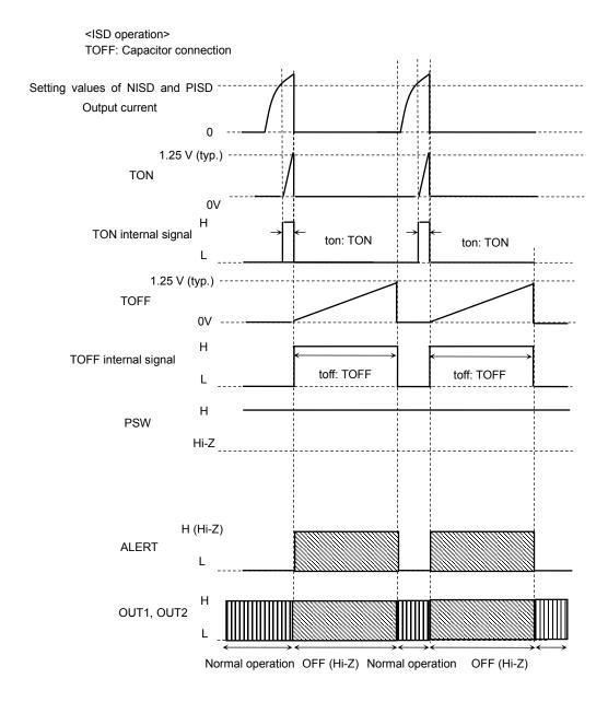
Note: The ISD circuit is activated if the absolute maximum current rating is violated. Note that the circuit is provided as an auxiliary only and does not necessarily provide the IC with a perfect protection from damages due to overcurrent caused by power fault, ground fault, load-short and the like.
