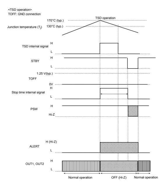
Note: The TSD circuit is activated if the absolute maximum junction temperature rating  $(T_j)$  of 150°C is violated. Note that the circuit is provided as an auxiliary only and does not necessarily provide the IC with a perfect protection from any kind of damages.
