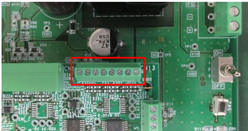
Figure 3-15 Pulse Train Command Connector
