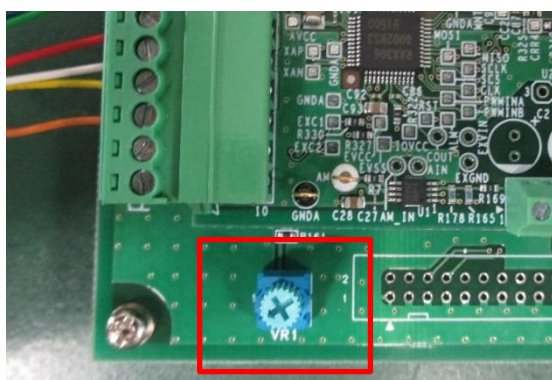
Figure 3-21 Location of the Variable Resistor
