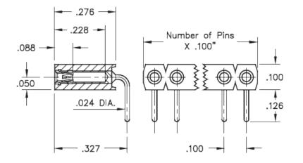
Interconnect Socket Right Angle Socket Accepts .025"- .037" (0,635 - 0,94 mm)dia leads Single Row Through Hole Plating Code: 93 Shell Plating: 200 μ" Tin/Lead(93/7) over 100 μ" Nickel Inner Contact Plating: 30 µ" Gold over 50 µ" Nickel
