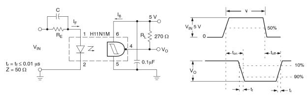
Figure 7. Switching Test Circuit and Waveforms
