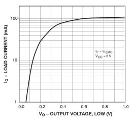
Figure 4. Load Current vs. Output Voltage
