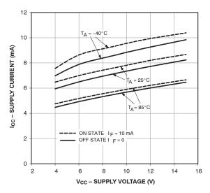
Figure 5. Supply Current vs. Supply Voltage
