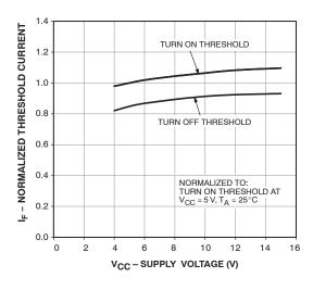
Figure 2. Threshold Current vs. Supply Voltage
