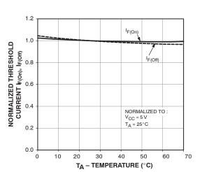
Figure 3. Threshold Current vs. Temperature
