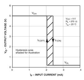
Figure 1. Transfer Characteristics
