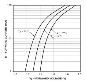
Figure 6. LED Forward Current vs. Forward Voltage
