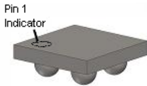
Figure 3. WLCSP Bumps Facing Down (Top View)
