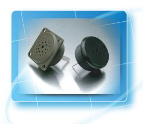
The SP27 standard buzzer is a small sized high quality buzzer to be used in applications where space is limited. The SP27 covers a wide range of applications, with an extremely high sound output of 94 dB(A) and a max. supply voltage of 9Vdc.
