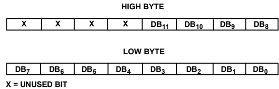
Figure 38. Data Format for AD5341
