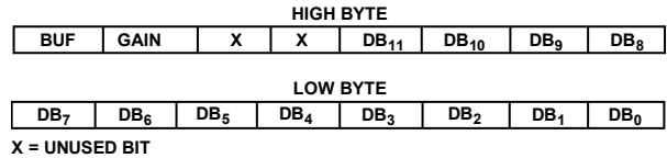
Figure 42. AD5341 with GAIN and BUF Data on 8-Bit Bus
