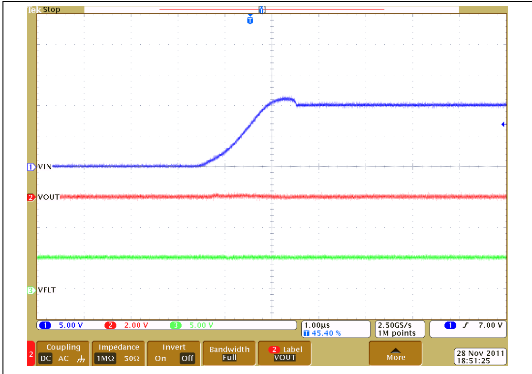
Figure 15. Startup to overvoltage (detail)
