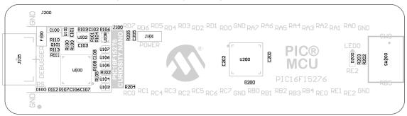
Figure 7-3. PIC16F15276 Curiosity Nano Assembly Drawing Bottom
