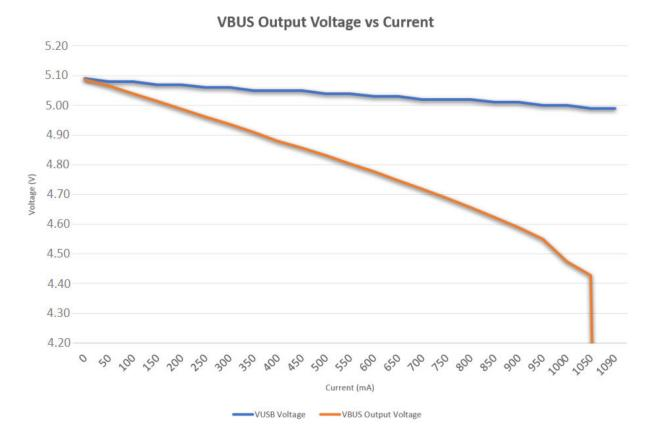
Figure 3-6. VBUS Output Voltage vs. Current
