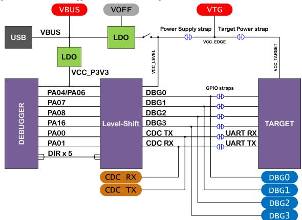
Figure 7-6. On-Board Debugger Connection Cut Straps
