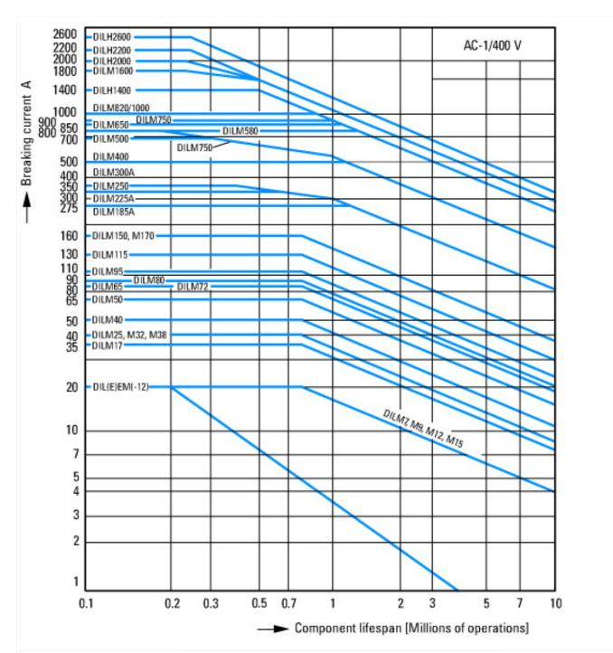
Switching duty for non-motor loads, 3-pole, 4-pole Operating characteristics
