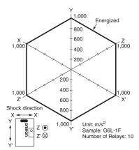
Conditions: Shock is applied in  $\pm X$ ,  $\pm Y$ , and  $\pm Z$  directions three times each with and without energizing the Relays to check the number of contact
