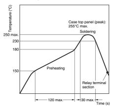
Note: The temperature profile indicates the temperature on the PCB.
