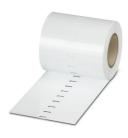
Marker for terminal blocks, Roll, white, unlabeled, can be labeled with: THERMOMARK ROLL 2.0, THERMOMARK ROLL, THERMOMARK ROLL X1, THERMOMARK ROLL MASTER 300/600, THERMOMARK X1.2, THERMOMARK S1.1, perforated, mounting type: snapped, snap into flat marker groove, for terminal block width: 6.2 mm, lettering field size:  $6.35 \times 6.15$  mm, Number of individual labels: 16000
