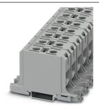
High-current terminal block, Terminal block for aluminum and copper conductors (AL-CU), nom. voltage: 1000 V, nominal current: 145 A, connection method: Screw connection, number of connections: 2, number of positions: 1, cross section: 6 mm² - 50 mm², AWG: 6 - 1/0, width: 19.2 mm, height: 51 mm, color: gray, mounting type: NS 35/15, NS 35/7,5
