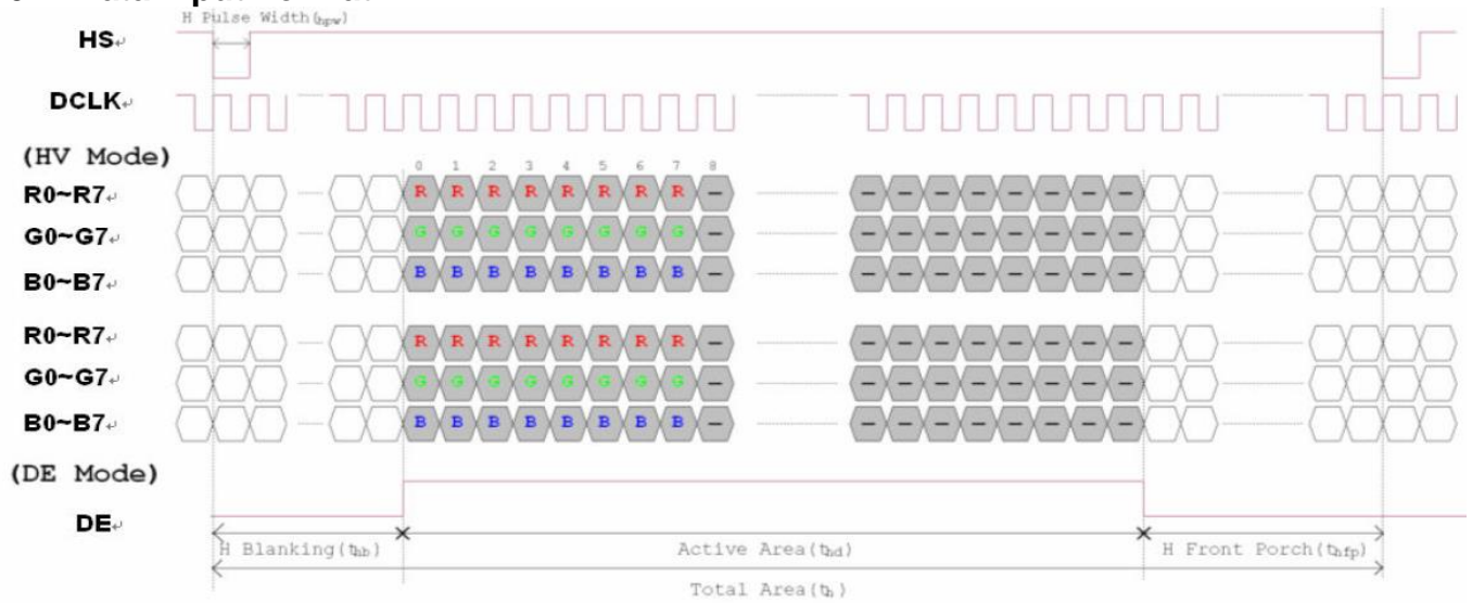
Fig1. Horizontal input timing diagram
