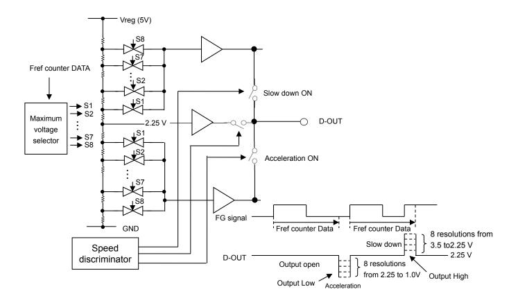
Fref counter DATA is changed depending on Fref frequency. Corresponding to this counter DATA, the peak voltage of D-OUT signal is switched as follows.
