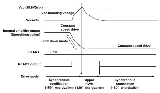
The maximum Vcc of the power supply voltage to be used in normal operation should be set VK = 27.8 V or less.
