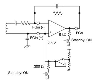
The FG amplifier supports a pattern FG and sets 2.5V of the reference voltage internally. The signal for the multiple of a gain is output by inputting sine wave more than 50 mVpp. The open loop gain is 40 dB (min) (@10 kHz, design target value).
