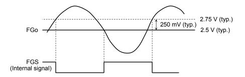
The dynamic range of FGo output is as follows. 1.2 V to V\_{reg} - 1.2 V at IFGo =  $\pm 100~\mu A$
