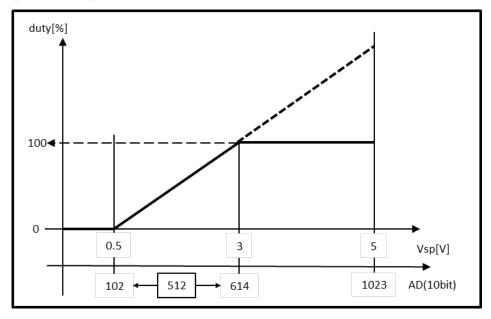
This circuit has 0.5V (typ.) of offset, and if the voltage of SP pin exceeds the value, an energization signal output operates. When the voltage of SP pin is 3.0V (typ.), the amplitude of internal modulation waveform (PWM duty of energization signal output) becomes maximum. When the voltage of SP pin is around 3V, the modulation waveform is output as the following image.
