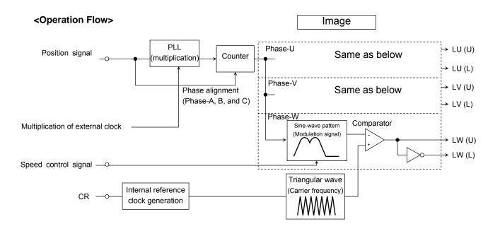
The modulation wave is generated by position detection signal. Sine-wave PWM signal is generated by comparing this modulation wave to triangular wave.
