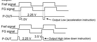
P-OUT is output in the timing of which motor rotation speed is in the stable area (READY = Low). The phase difference between Fref signal and FG signal is output.
