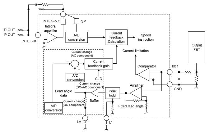
The current feedback gain is set with the CLD voltage.
