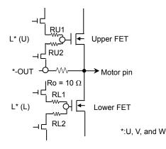
Note: Ro =  $10\Omega$  should be surely inserted between each OUT pin and the motor pin.
