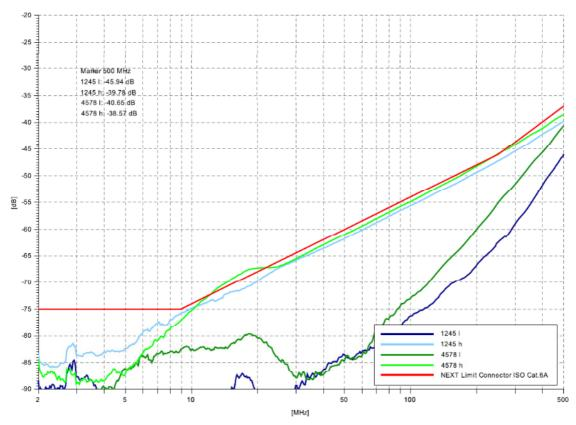
The results of the pairs 4578 seem to be below the limits in the frequency range of 10 to 20 MHz. However, this is a snapshot of an instantaneous signal trace frozen in time. Very low signal levels below 65 dB are susceptible to small changes in the physical arrangement of DUT and fixture. In this sense the limit line is not really violated. Furthermore, in this very low frequency range there is ample headroom to the channel specifications. Please note that most critical is NEXT above 250 MHz.
