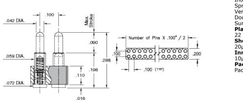
Description: Interconnect SLC Header Spring-Loaded Header Vertical Mount SMT Double Row Surface Mount Plating Code: 22 Shell Plating: 20μ" Gold over 100μ" Nickel Inner Spring Plating: 10μ" Gold Packaging: Packaged in Bulk
