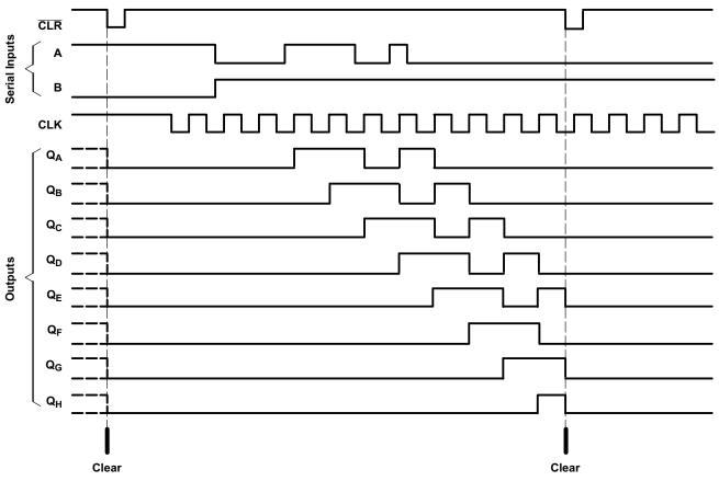
Figure 1. Typical Clear, Shift, and Clear Sequences
