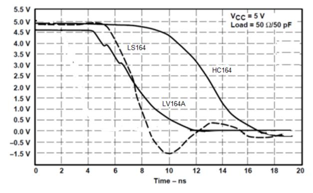
Figure 7. Switching Characteristics Comparison
