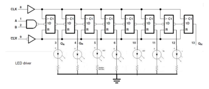
Figure 6. Typical Application Schematic
