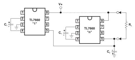
Figure 5. Paralleling Devices
