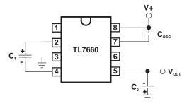
Figure 8. Lowering Oscillator Frequency
