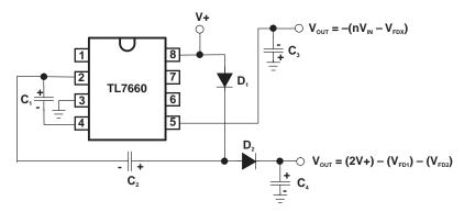
Figure 10. Combined Negative-Voltage Converter and Positive-Voltage Doubler
