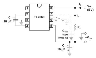
A. In the circuit, there is no external capacitor applied to terminal 7. However when device is plugged into a test socket, there is usually a very small but finite stray capacitance present on the order of 10 pF.
