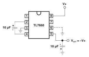
Figure 3. Simple Negative-Voltage Converter
