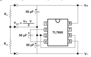
Figure 11. Splitting a Supply in Half
