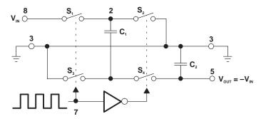
Figure 2. Idealized Negative-Voltage Converter
