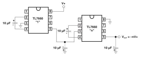
Figure 6. Cascading Devices for Increased Output Voltage
