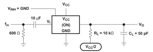
Figure 11. Sine-Wave Distortion
