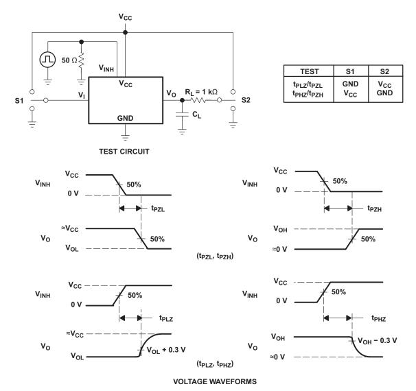
Figure 6. Switching Time (t<sub>PZL</sub>, t<sub>PLZ</sub>, t<sub>PZH</sub>, t<sub>PHZ</sub>), Control to Signal Output
