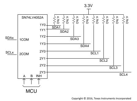
Figure 13. Typical I<sup>2</sup>C Multiplexing Application
