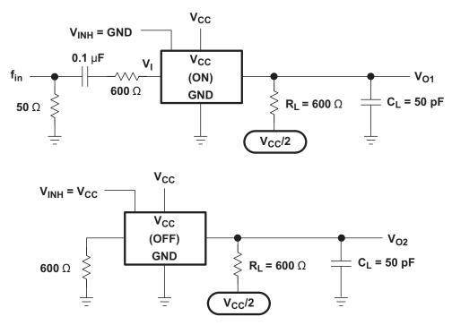
Figure 8. Crosstalk Between Any Two Switches
