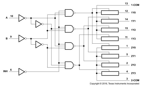
Figure 12. Logic Diagram (Positive Logic)
