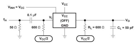
Figure 10. Feedthrough Attenuation (Switch OFF)
