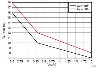
Figure 14. Maximum Propagation Delay vs V<sub>cc</sub>
